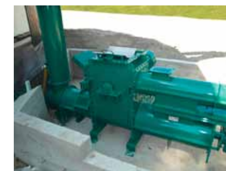
Shredder integrated in the conveyor system
