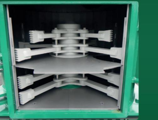
HPZ 900 rotor with patented intermediate floor.
