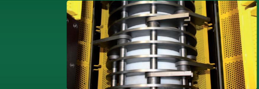
Robust hammer mechanism with lateral screen baskets to obtain a defined degree of separation in preparation for hygienisation
