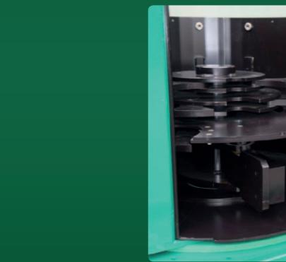
HPZ 1200 rotor with patented intermediate floor
