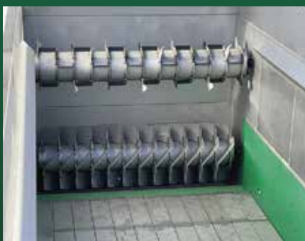
Alternatively: Break-up by rollers with tools instead of a mixing star
