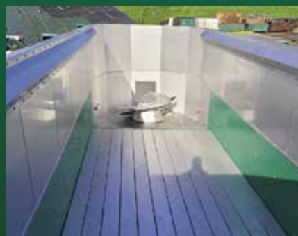
Surfaces in contact with substrate made of stainless steel or with plastic cladding
