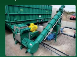
The patented Optimatic Hammer Mill can be flexibly integrated into the solids feeding system by means of a bypass. Substrates are force fed into the milling chamber, ensuring reliable, continuous feeding into the working chamber of the machine. Oscillating hammers or cutters in the rotor ensure a high tolerance for impurities. An optional lateral stator with spring-loaded counter knives provides optimal results, especially when milling
