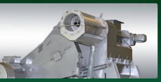
Spiral conveyor for discharge of packaging material
