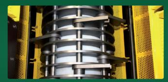
Robust hammer mechanism with lateral screen baskets to obtain a defined degree of separation in preparation for hygienisation
