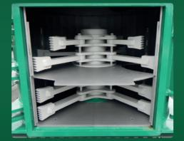
HPZ 900 rotor with patented intermediate floor.
