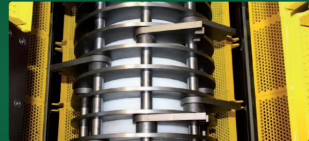
Robust hammer mechanism with lateral screen baskets to obtain a defined degree of separation in preparation for hygienisation
