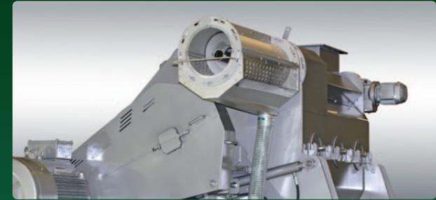
Spiral conveyor for discharge of packaging material
