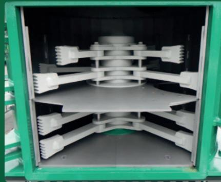
HPZ 900 rotor with patented intermediate floor.
