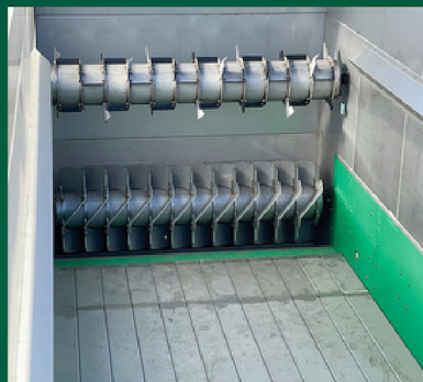
Alternatively: Break-up by rollers with tools instead of a mixing star.
